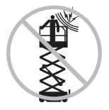
Keep away from the machine if it contacts energized power lines. Personnel on the ground or in the platform must not touch or operate the machine until energized power lines are shut off. Do not operate the machine during lightning or storms.
