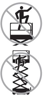
Do not sit, stand, or climb on the platform guard rails. Maintain a firm footing on the platform floor at all times.
