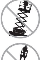
Do not raise the platform unless the machine is on a firm, level surface.
