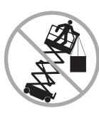
Do not place or attach fixed or overhanging loads to any part of this machine.
